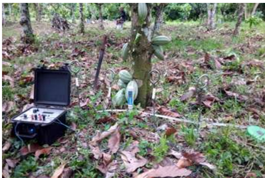
Plate 1: A set up of soil electrical resistivity and soil moisture survey under cocoa plantation in-situ
