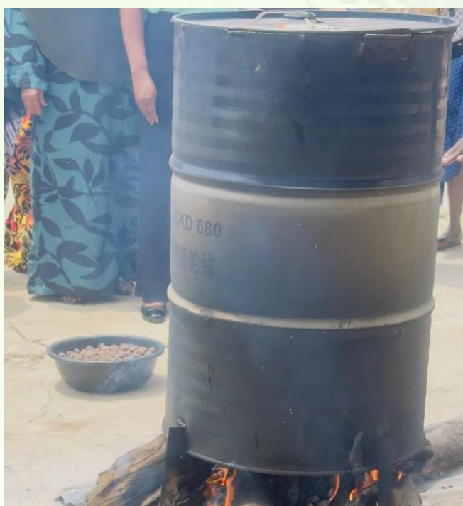
Fabricated cashew nut boiler used during the training
